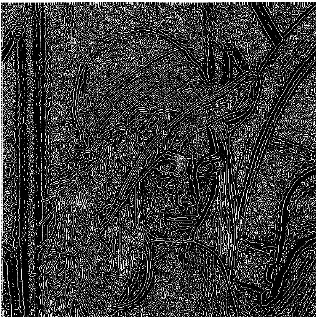
Figure 7: edge detected from the local maxima of the wavelet transform modulus, at the scale 2^2 .
