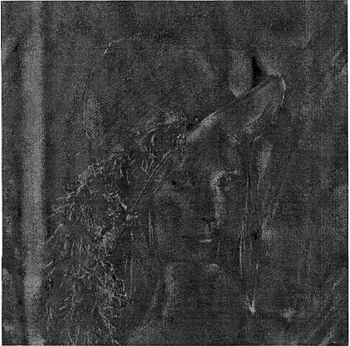
Figure 10: this error image is obtained by subtracting the edge coded image of Fig. 9 from the original image in Fig. 6. Black, grey and white pixels correspond respectively to negative, zero and positive coefficients. Most of its energy is concentrated in texture regions.
