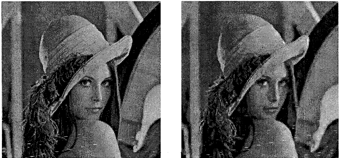
Figure 15: Left: original image. Right: image obtained by adding the coded error image at the right of Fig. 14 with the coded edge image of Fig. 5. This image was coded on 0.202 bits per pixel.
