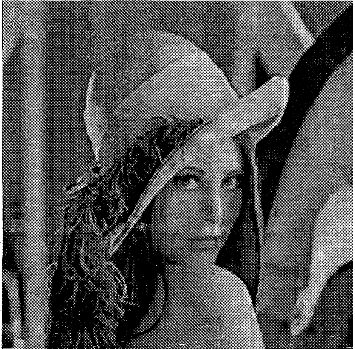
Figure 13: coded image obtained by adding the edge coded lady image of Fig. 9 and the error coded image of Fig. 12. This image is coded on a total of 0.081 bits per pixel.
